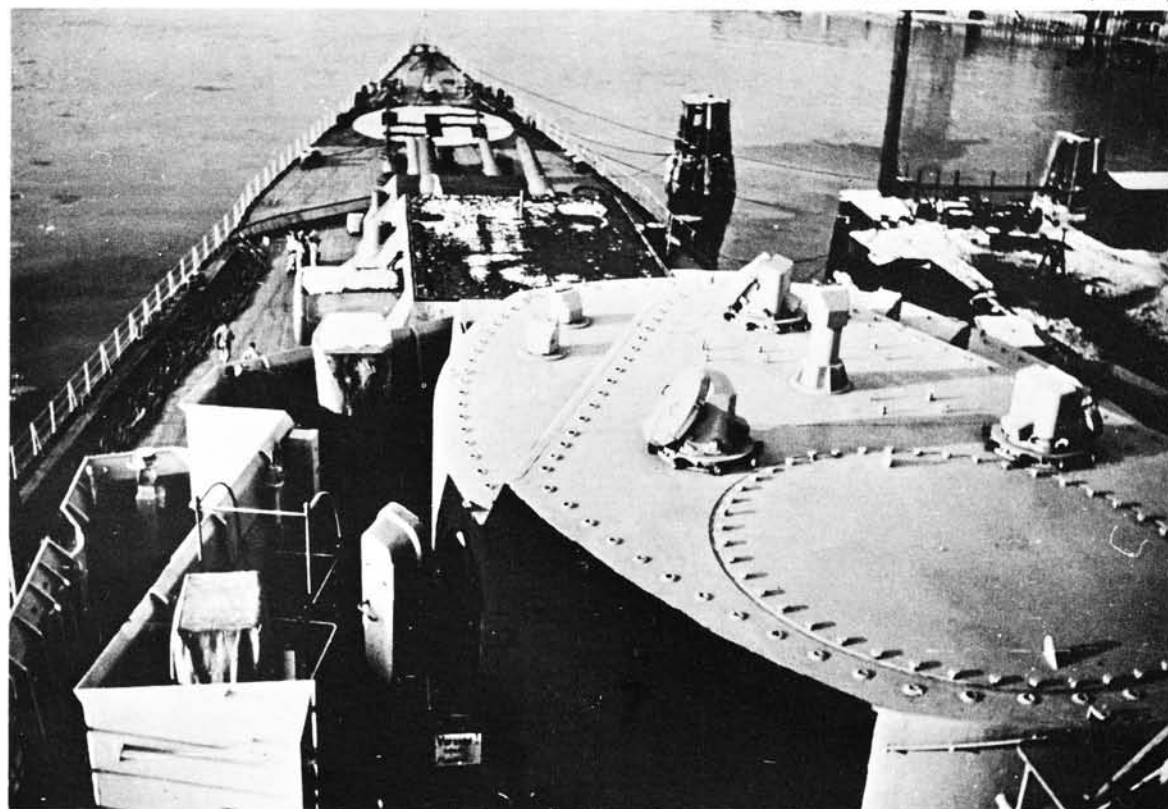
Fo'c'sle with command tower from outside the admiral's bridge. In addition, wings of bridges are visible. Note the assembly hatch for the instruments in the roof of the command tower and also armoured access door
