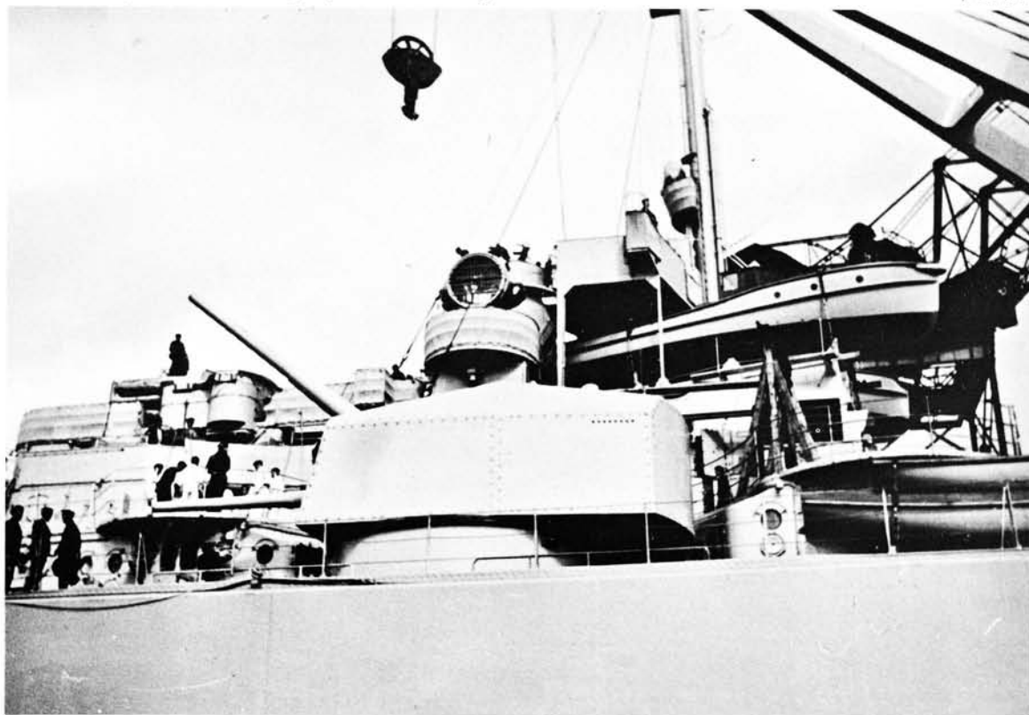
The after 15cm twin turret, after superstructure, searchlight and boat stowage. The recently installed 3.7cm guns are just visible on the sponson behind the group of men. Hamburg 1940 (Author)
